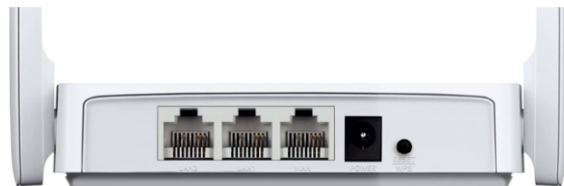
LAN Ports WAN Port Power WPS/Reset Connect to desktops, game consoles, etc. Connect to the Internet
