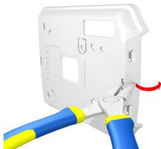
Figure 2: Surface-mount cabling plastic tab removal
