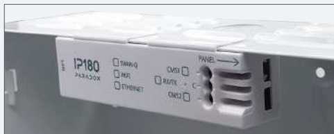
IP180 Installed in a Metal Box
